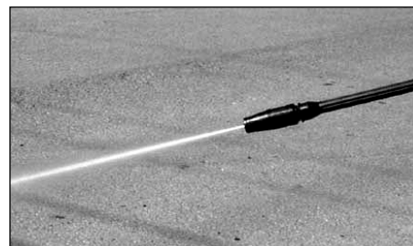
Figure 13 - Narrow high impact stream
